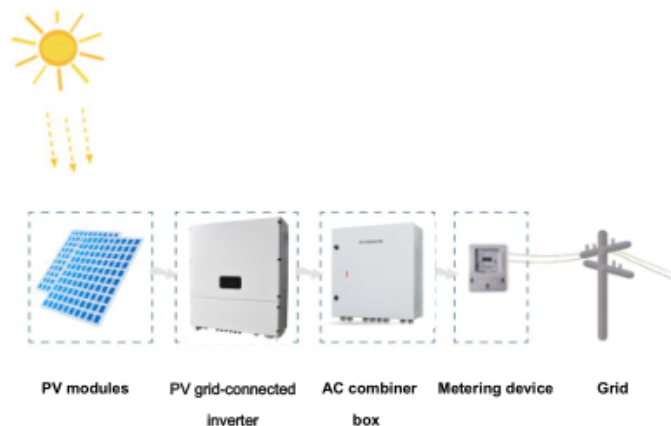
Fig. 1 PV grid-connected power generation system
